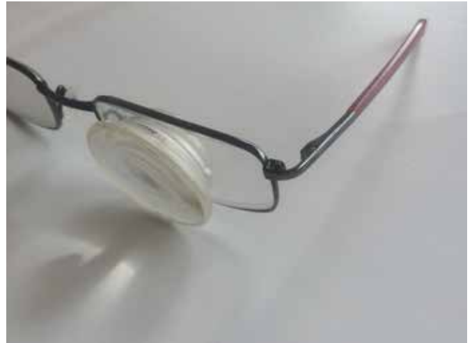
Two lenses in combination with anti-reflection treatment on all four surfaces produces the least amount of optical errors.
